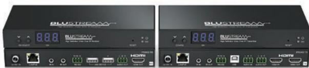
The IP50HD is an industry leading 1080p video over IP solution that uses H.265 compression technology to deliver HDMI, Bi-directional IR, RS-232 & USB/KVM up to lengths of 100m over standard network architecture. The products can be powered via PoE from the network switch or locally should the switch not support PoE. With multiple configuration options available the Multicast HD solution is ideal for large scale education installations.
