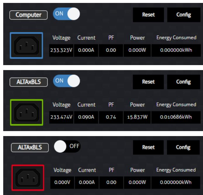
When an outlet of the PWR4IEC enters a warning state, the outlet will be turned off and highlighted in red. This is triggered by abnormal voltage or current on the outlet. When attempting to power on the outlet, a warning dialog will be shown allowing for the warning to be cleared and the outlet to resume normal operation:
