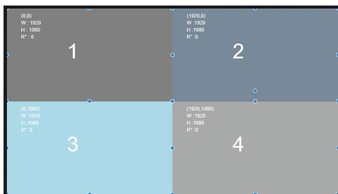
With the default 2 x 2 Video Wall loaded, select one of the windows, and turn off its active toggle.
