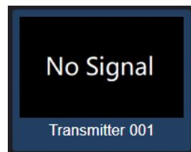
If the Receiver preview shows 'No Signal', the device may not be powered or connected to the AVoIP system. Confirm that the Receiver is online and linked to a functioning Transmitter.
